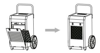
Insert the filter box then close the wind panel.
